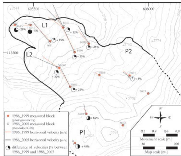
Figure 1: Mean annual horizontal movement [m a<sup>-1</sup>] on BBrg for the time period 1986-1999 (photogrammetry) and 1986-2005 (theodolite-GPS). Dots show the initial position of “photogrammetric” and “geodetic” boulders used for comparison (they may be different).
