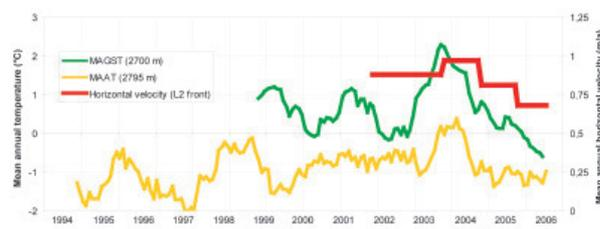
Figure 2: Comparison between MAGST [°C] MAAT [°C] and mean annual velocities [m a<sup>-1</sup>] on front of L2.
