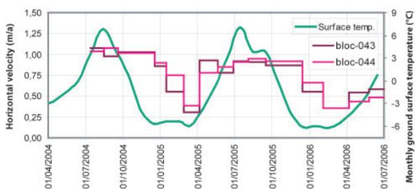
**Figure 4:** Seasonal variations of horizontal velocities [ $\text{m a}^{-1}$ ] (Juno4-Julo6) of boulders 43 and 44 placed on the front of L2 and ground surface temperature ( $^{\circ}\text{C}$ ).
