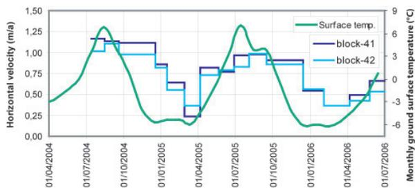
**Figure 3:** Seasonal variations of horizontal velocities [ $\text{m a}^{-1}$ ] (Juno4-Julo6) of boulders 41 and 42 placed on the front of L2 and ground surface temperature ( $^{\circ}\text{C}$ ).
