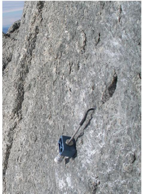
*Photo 6: M-Log4 data logger installed in a rock face. The body of the logger is held by two hydraulic hose brackets (blue) and two screws anchored in wall plugs. Photo: S. Gruber.*
