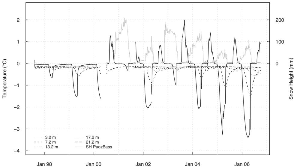
Fig. A.26: Temperature-time-plot of the borehole Schaefberg-Pontresina 02/90 for the thermistors at 3.2, 7.2, 13.2, 17.2, and 21.2 m depth. Additionally, the snow height at Puoz Bass is displayed.
