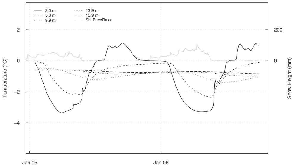
Fig. A.25: Temperature-time-plot of the borehole Schaefberg-Pontresina 01/90 for the thermistors at 3.0, 5.0, 9.9, 13.9, and 15.9 m depth. Additionally, the snow height at Puoz Bass is displayed.
