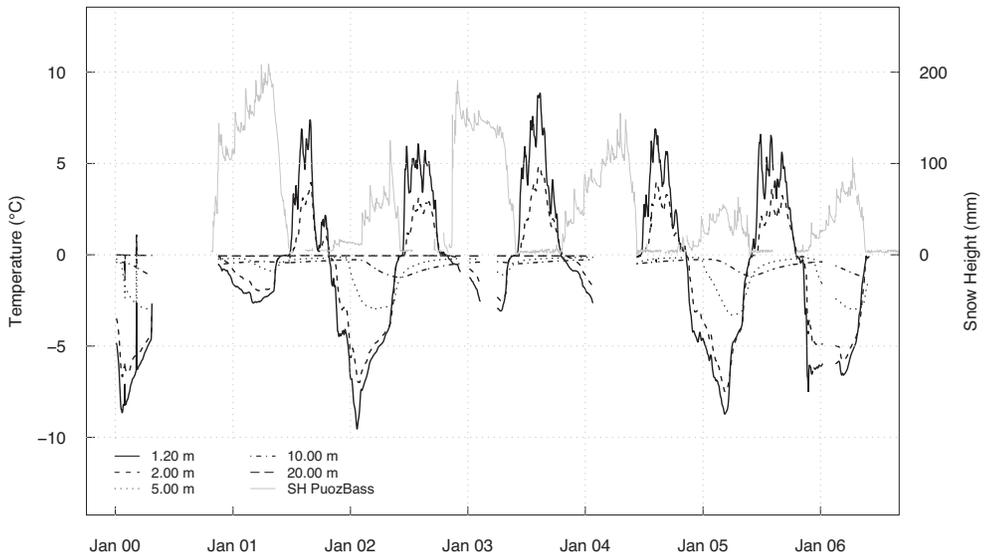
Fig. A.18: Temperature-time-plot of the borehole Muragl 04/99 for the thermistors at 1.2, 2.0, 5.0, 10.0, and 20.0 m depth. Additionally, the snow height at Puoz Bass is displayed.
