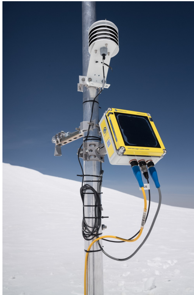
Figure 9: detail of the monitoring station with air thermometer (top), sonic ranger (left) and data logger (right). The yellow cable leads to the thermistor chain. Image ©Horst Machguth.
